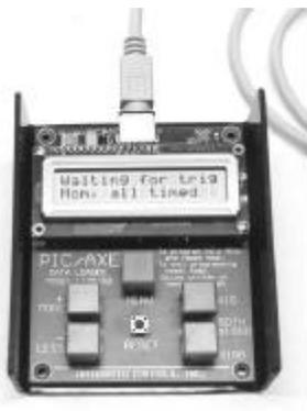
The PIC/AXE program data loader is an optional hand held accessory with switches and an LCD Display and is used to program the various time and level settings. Once programmed with the PIC/AXE (or at the factory) the L129 is a stand-alone controller. The PIC/AXE can also function as a remote control in Run mode.
